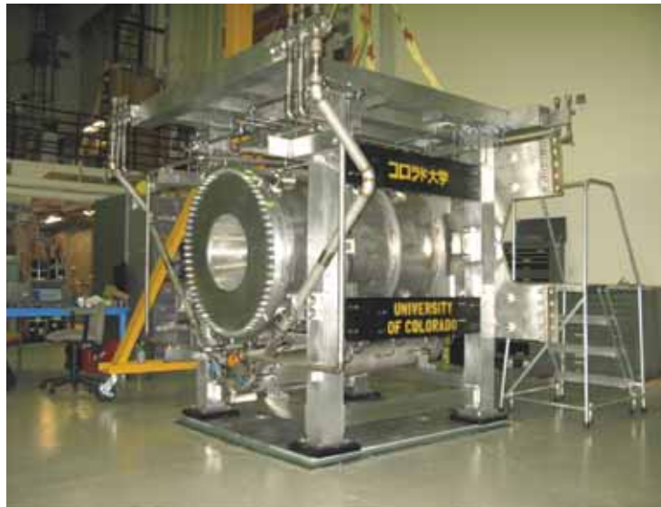
One of the three focusing ‘horns’ now operating on T2K that was designed and built by the CU research team.
