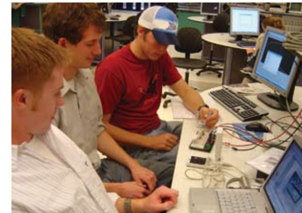
The Intel senior design team performs tests to characterize new thermal electric modules from Intel. The team developed an entire test system and efficient test methodology for these thermal electric devices.
