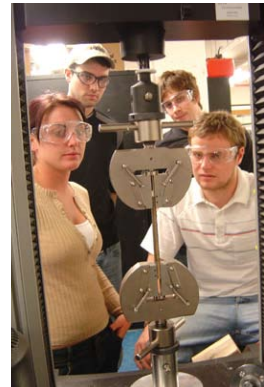
The Composite Technology Development senior design team performs tests to characterize a new shape memory polymer material for which they are investigating product applications.
