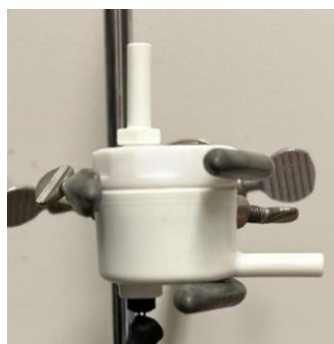
Figure 2. UV LED reactor used in bench scale system testing the efficacy of inactivating planktonic cells prior to biofilm formation.
