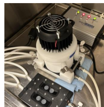
Figure 3. Bench scale experimental system testing the impact of constant, direct UV irradiation in disrupting biofilm formation.
