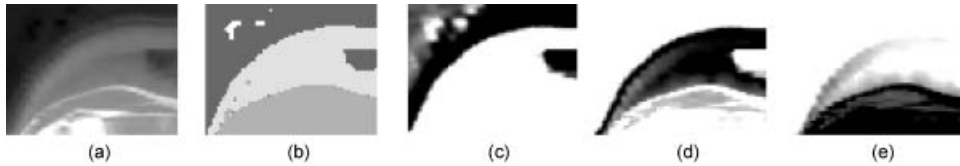
Figure 19. Elevation and results of crisp and fuzzy classification: (a) DEM of Ameland for the year 1995, (b) crisp classification of elevations, (c) vague shore, (d) vague beach, (e) vague dune. Saturated colour shows high membership for vague objects.
