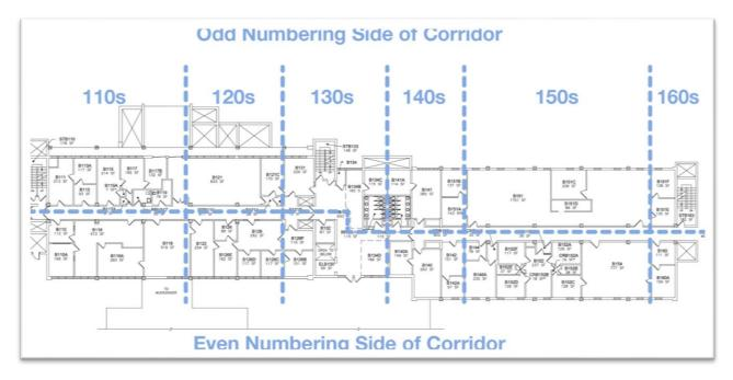
This first floor level plan represents a typical building with one central corridor bisecting the two halves of the layout. Refer to this image throughout the discussion on room numbering.
