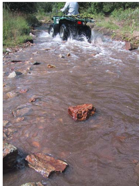
EVEN graduate Durelle Scott (the headless rider) drives an ATV in a flooded road near a creek to simulate the generation of suspended sediment by off-highway vehicle recreation.
