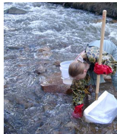
Susan Bautts, an EVEN graduate, collects samples of the benthic macroinvertebrate population in an acid mine drainage-affected stream.
