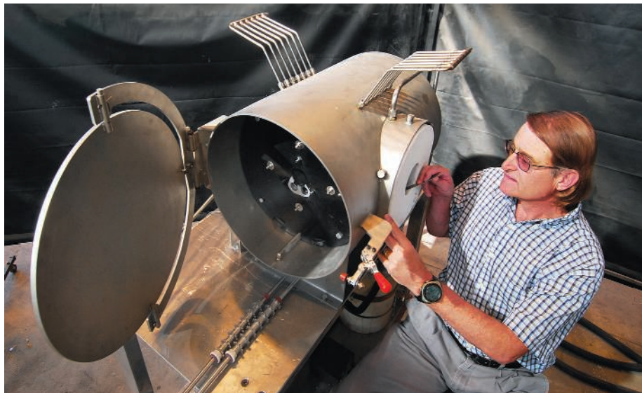
Re-energize. Solar engineer Richard Diver of Sandia helped develop this reactor, which uses heat from concentrated sunlight to split water into hydrogen and oxygen, and carbon dioxide into carbon monoxide and oxygen.
