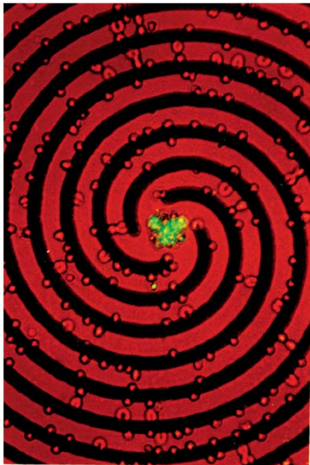
Fig. 11. Cell trapping and focusing on a spiral traveling wave DEP electrode. Fluorescently labeled human erythrocytes infected by the malarial agent Plasmodium falciparum have been discriminated from uninfected cells and focused from a scattered state to the center of the spiral electrode.
