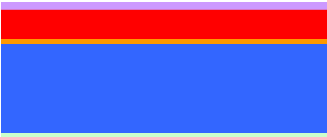
FIGURE 1.3. A phosphosilicate glass layer (PSG) is deposited, and the wafers are annealed at 1050 ^{\circ} C for 1 hour in Argon to drive the Phosphorous dopant into the top surface of the Silicon layer. The PSG layer is subsequently removed using wet chemical etching.
