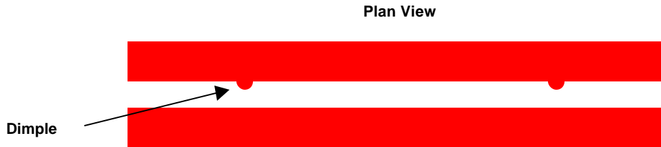
FIGURE 2.4.4. Example of dimple features in the SOI Mask level to reduce lateral stiction affects during release.
