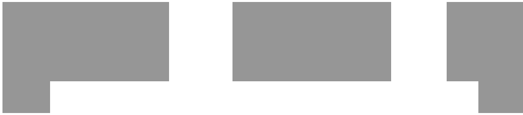
FIGURE 1.8. A separate silicon wafer is used to fabricate a shadow mask for the Metal pattern. Standoffs are pre-fabricated into the shadow mask so that the shadow mask does not come into contact with patterned features in the Silicon layer of the SOI wafer. The shadow mask wafers are then coated with photoresist and the fourth level (METAL) is lithographically patterned. DRIE silicon etching is used to etch completely through the shadow mask wafer, producing through holes for the Metal to be evaporated. After the etch is completed, the photoresist is removed
