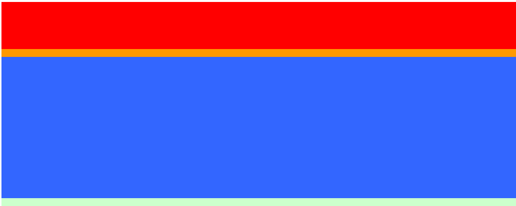
FIGURE 1.2. The SOI wafers consist of a 10 \mu m Silicon layer, a 1 \mu m Oxide layer, and a 400 \mu m Substrate layer. A Bottom Side Oxide layer is also initially present on the wafers.
