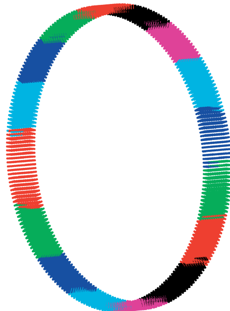
Fig. 8 Free-free ring modeled by solid elements.
