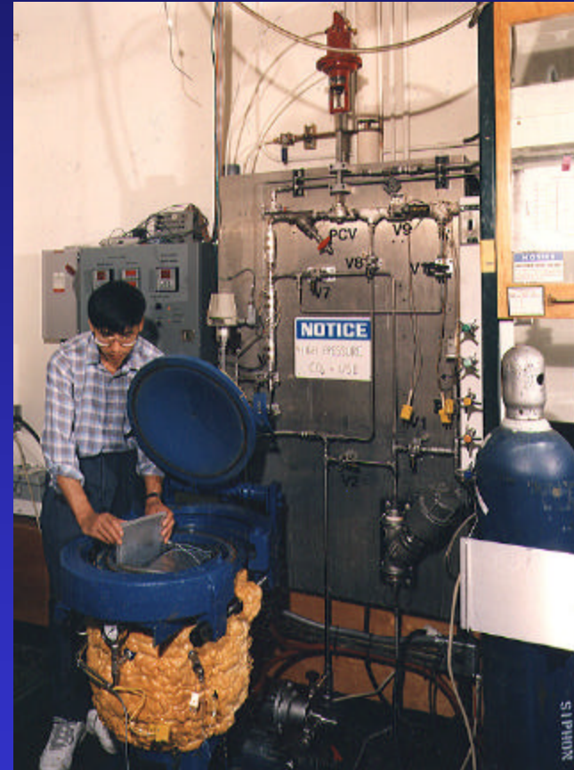
Supercritical Drying System - 40 L capacity, square gels 28 cm per side Berkeley National Labs
