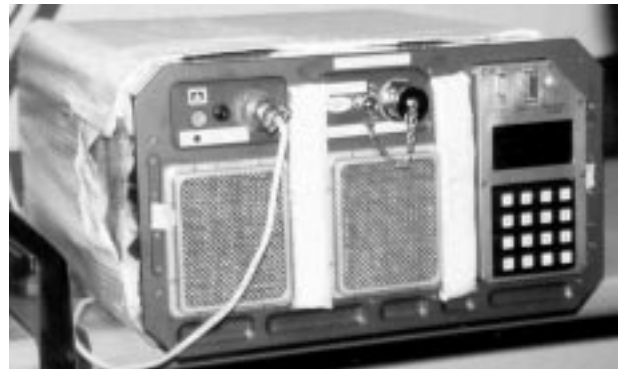
Figure 5. Air inlet, air outlet and computer interface of the Isothermal Containment Module (ICM-V2), a middeck locker insert incubator (6°C → 37°C).
