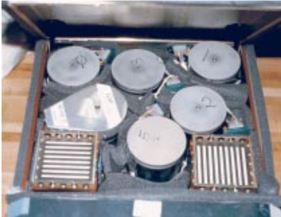
Figure 6. Incubator filled with experimental samples for the STS-95 flight. To avoid thermal gradients across the incubator volume, all walls are water cooled and material thickness of sample containers are increased to provide thermal pathways.
