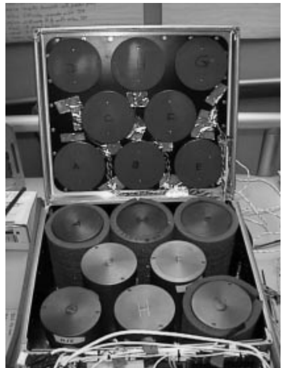
Figure 8. Incubator with 8 individually controlled sample containers. Each container has its own, independent proportional temperature controller and heat pump, allowing 8 different temperature environments simultaneously on the same space flight in the same incubator.
