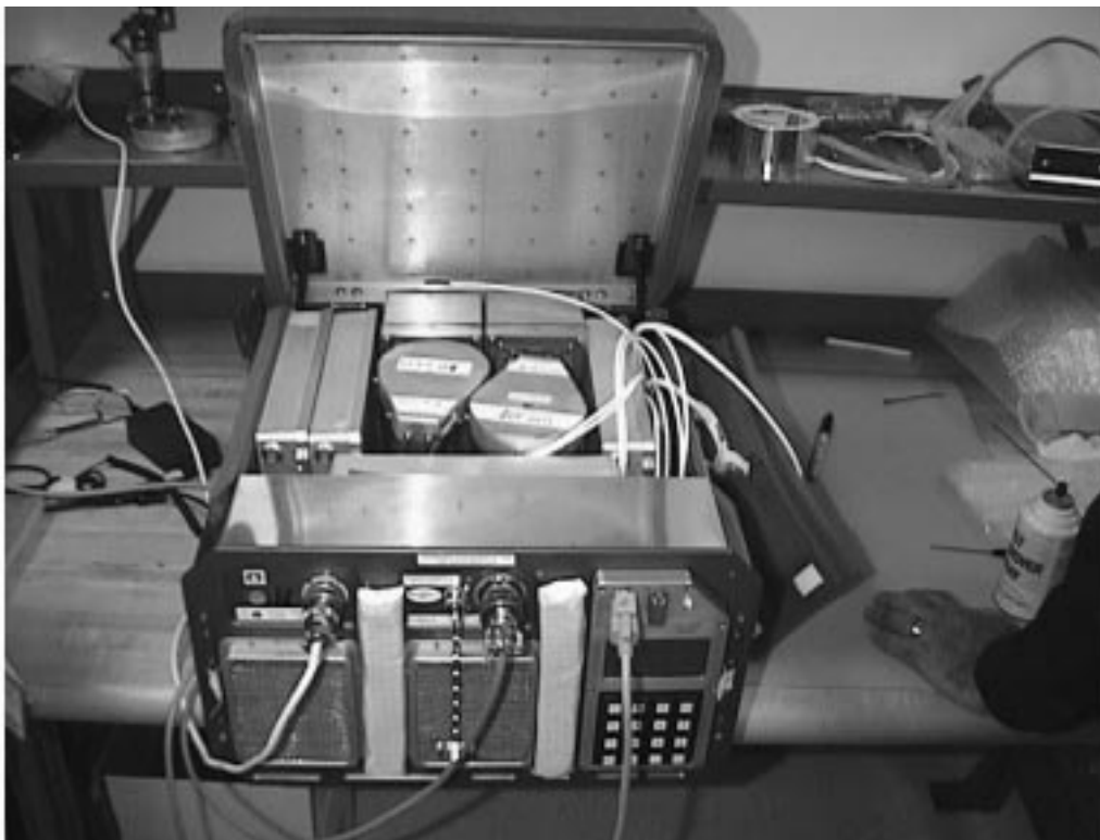
Figure 9. The CGBA Hardware Complement, showing the ICM incubator and a variety of potential experiment sample containment hardware. Samples can be contained inside the Fluid Processing Apparatus (FPA) and the Group Activation Pack (GAP) sample containment hardware. GAPS are automatically activated with a motor drive (Auto-GAP) once on orbit. Examples of other experiment-specific containment hardware include the Gas Exchange Fermentation Apparatus (GEFA – liquid and solid fermentation), the Illuminated Culture Vessel (ICV – plant tissue cultures under red LED light), and the automated BioSpace Protein Crystallization System (BPCS). All sample containers (GAP, FPA, ICV, GEFA, BPCS) are stored inside the temperature-controlled Isothermal Containment Module (ICM) cooler / incubator facility. The individual experiment assemblies are controlled using an RS-485 multidrop control network.
