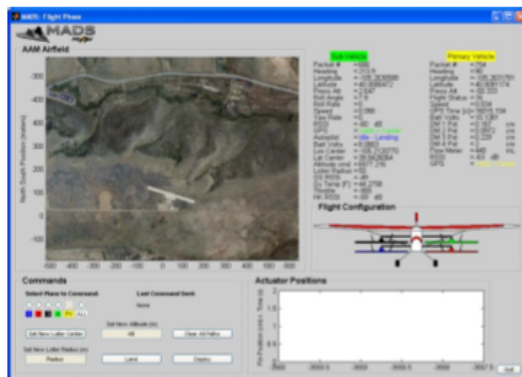
Figure 9. Second screen available to the user in the ground station GUI.
