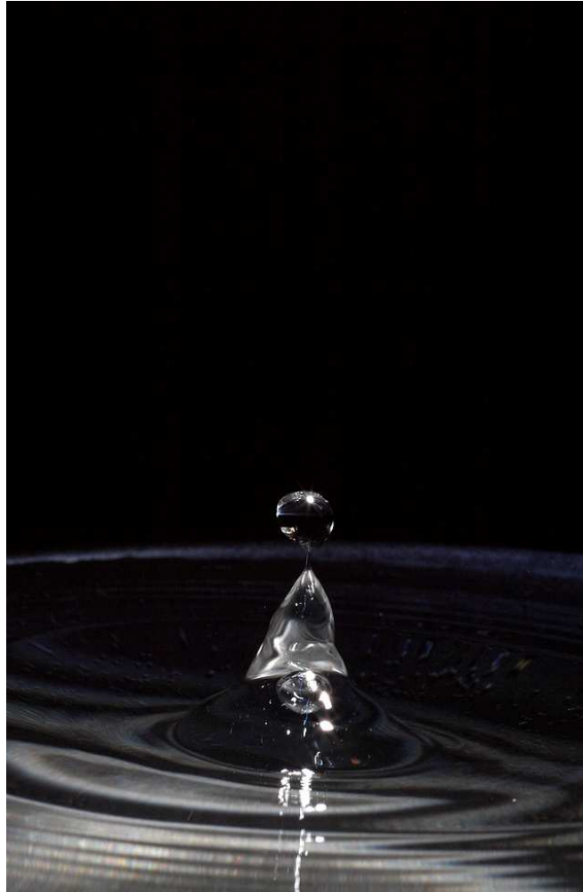
Fig. 3. Strobe image of a Worthington jet after the impact of a water droplet. Mark Donohue, Luciano Mazzaro, Blake Nolan, Tait Stangl, by permission.
