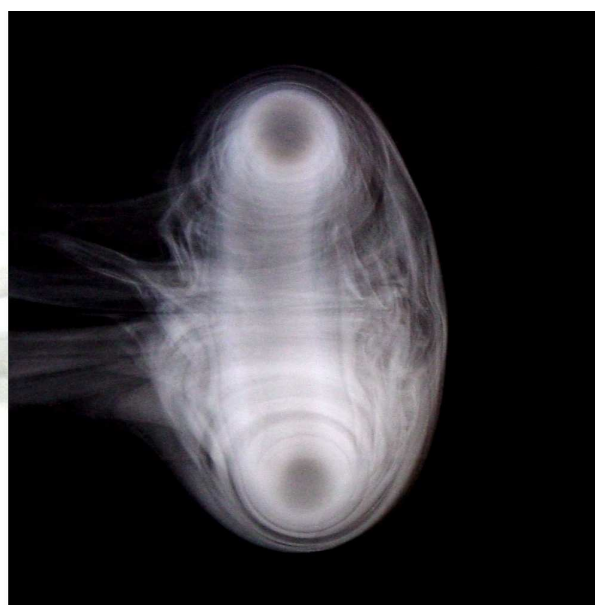
Fig. 7. Vortex ring in air, visualized with stage smoke. Emrys Hall, Thomas King, Bethany Rotherham, Brynne Sutton, by permission.
