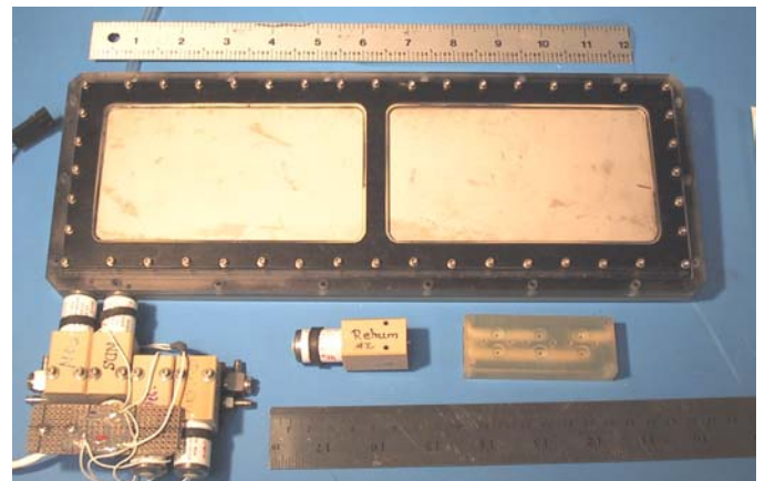
Figure 9 PGBA Humidity control porous plate (0.2 \mu m media grade), with 50 \mu L/stroke fixed volume piston pumps, pump manifold and individual pump and manifold.
