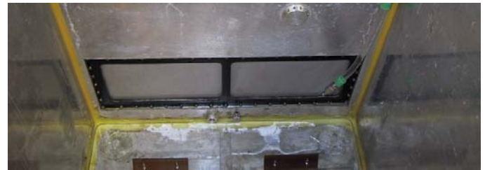
Figure 8. PGBA humidity control porous plate (0.2 \mu m media grade) inside the sealed plant chamber (plant insert removed).
