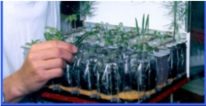
Figure 1. The PGBA root zone hydration system (Hoehn et al., 1998). Media for each plant is contained in gas-permeable polypropylene bags. The bags reduce evaporation, while maintaining proper root zone oxygenation. Each bag is surrounded by airflow passage ways. The bags are resupplied from the bottom with condensate from the humidity control system (App. 1).
