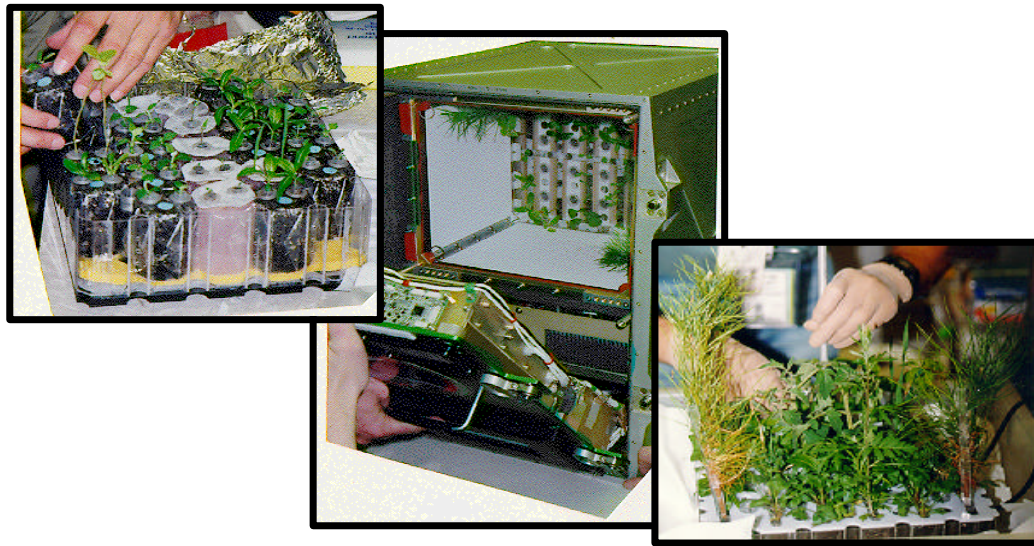
Figure 1: The PGBA spaceflight plant growth chamber as flown aboard STS-83. The plant roots are contained in soil (water replenishment) or agar media (no water replenishment, Heyenga, 1997). The plant chamber is sealed from the crew cabin, but receives CO 2 -rich cabin air for controlled CO 2 replenishment (Hoehn et al., 1997). (Left) Root tray, (Center) sealed plant chamber and lighting / video system, (Right) plants grown in space flight during STS-83.
