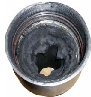
Figure 6: Eroded Castable Ceramic Nozzle
