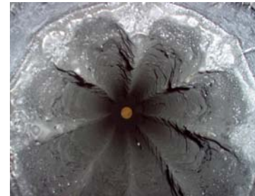
Figure 9: 5000 lb f fuel grain post-fire
