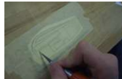
Figure 9. Wing mold and release strips
